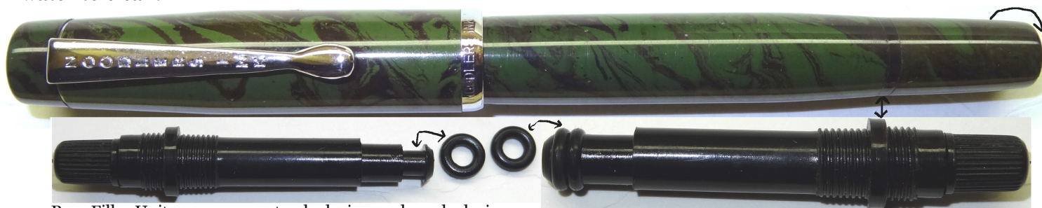
Rear Filler Unit -remove counterclockwise, replace clockwise
